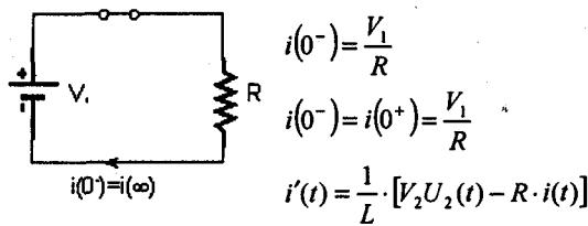
$$i'(0^+) = \frac{1}{L} [V_2 - R \cdot i(0^+)] = \frac{V_2}{L} - \frac{R}{L} i(0^+)$$
