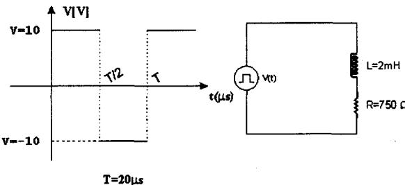
$$A_0 = 0 \text{ ve } A_n = 0 \text{ iken } B_n = \frac{2}{T} \int_0^T V \sin n\omega t dt = \frac{2V}{n\pi} (1 - \cos n\pi)$$
