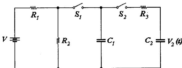
$$\begin{aligned} R_1 &= 10k & V &= 30V_{dc} \\ R_2 &= 20k & C_1 &= 10\mu F \\ R_3 &= 10k & C_2 &= 20\mu F \end{aligned}$$
