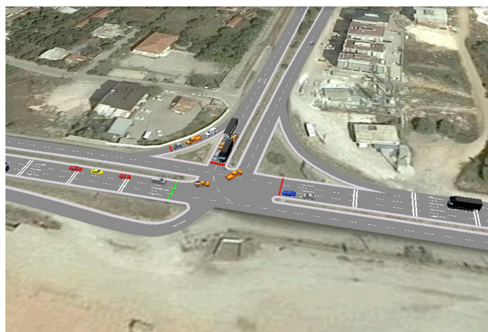
Figure 2. The 3D model of the intersection number 9 was shown in PTV Vissim.
